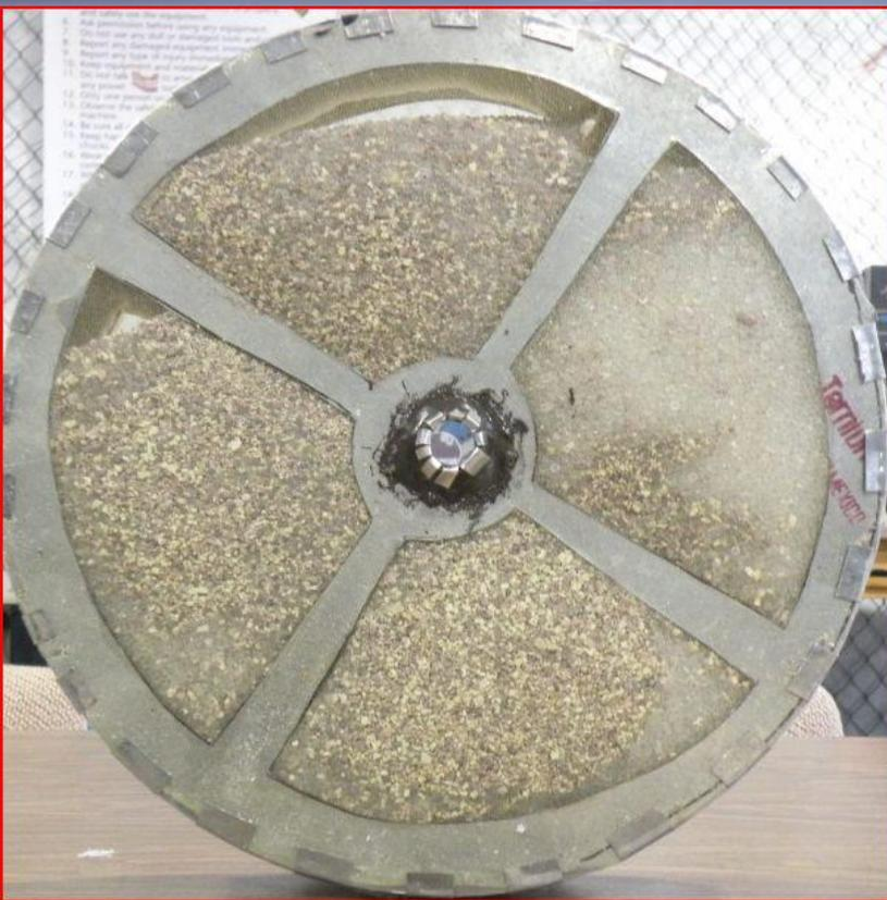
Desiccant Wheel filled up with Silica Gel.
