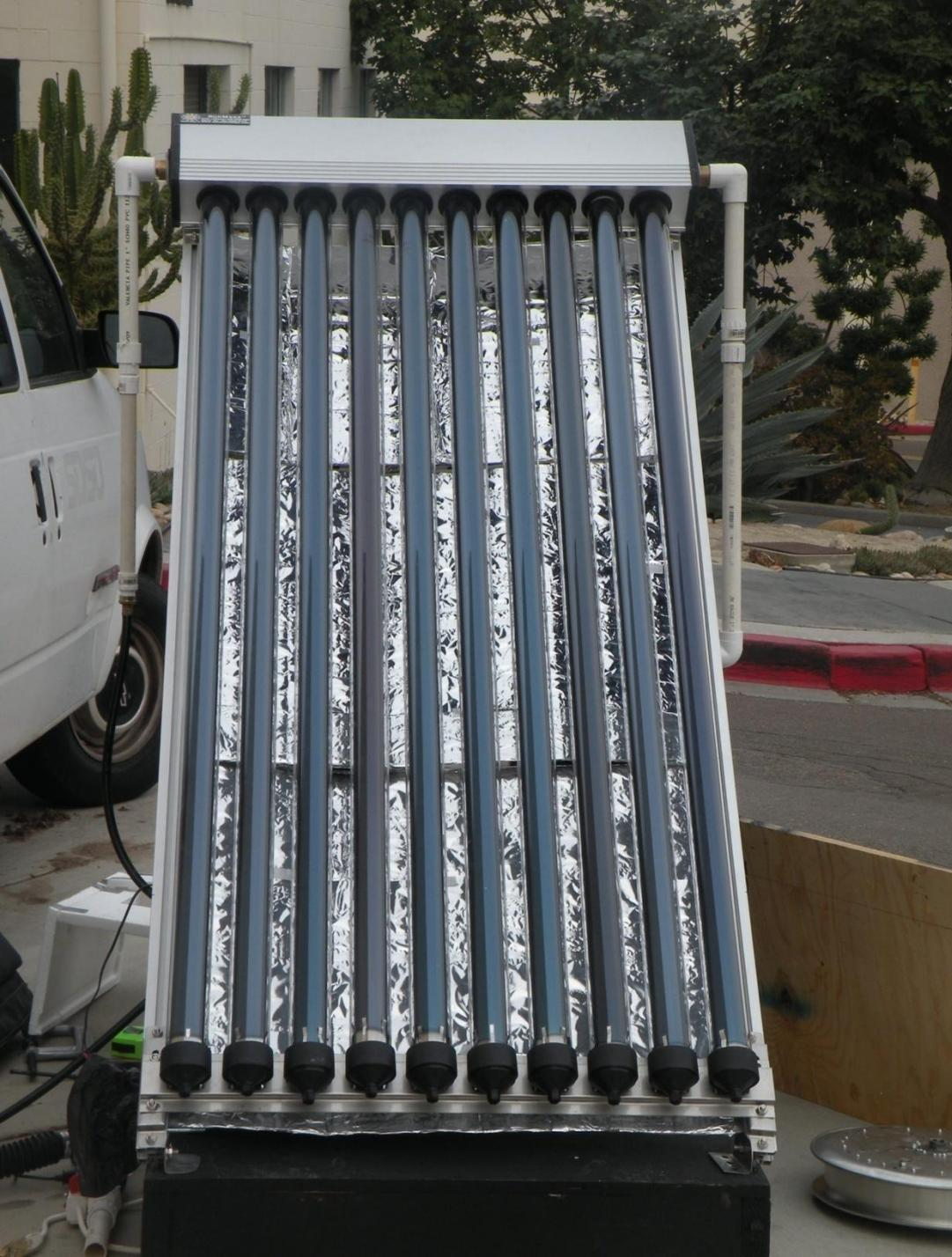
Aluminum sheets were added behind the tubes to maximize solar heating capacity.
