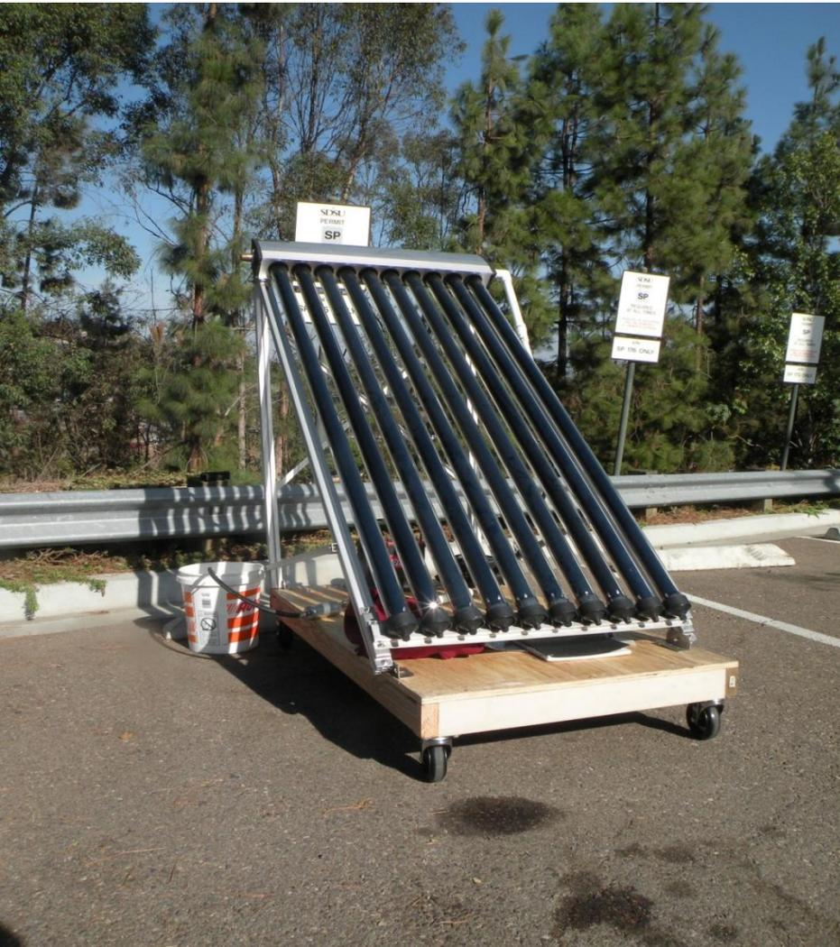
Set-up to test the attainable temperatures of water through the solar collector.
